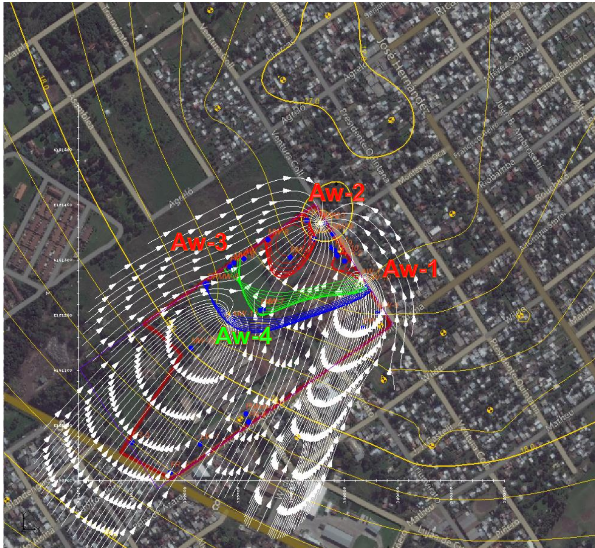
Modeled optimized Pumping rate - Mean Water Table Conditions 3-D Groundwater Flow Model Version 5
